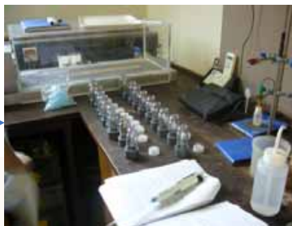
Soil samples are weighed into centrifuge tubes
