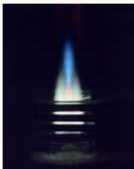
Samples are analysed by ICP-AES
