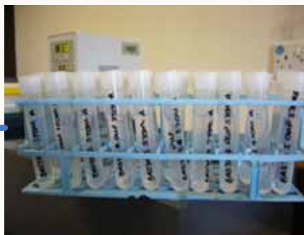
Decanted samples are diluted and preserved in 0.1 M HNO 3
