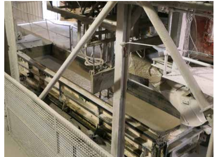
Liquid batched slurry mix at Mannock Aircrete.
