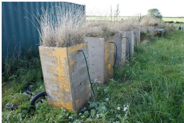
Figure 8. Site lysimeters with water content measurements and grass roots monitoring, next to the Bionicle experimental embankment
