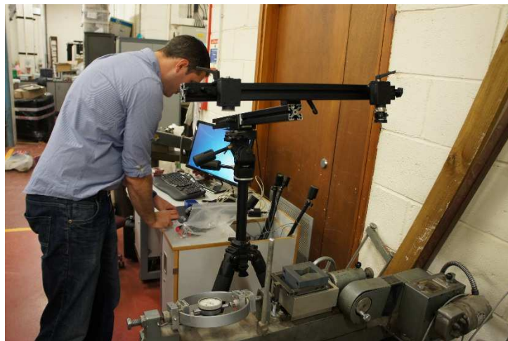
Figure 2. Preparation of the digital image correlation (DIC) system by Dr Stirling
