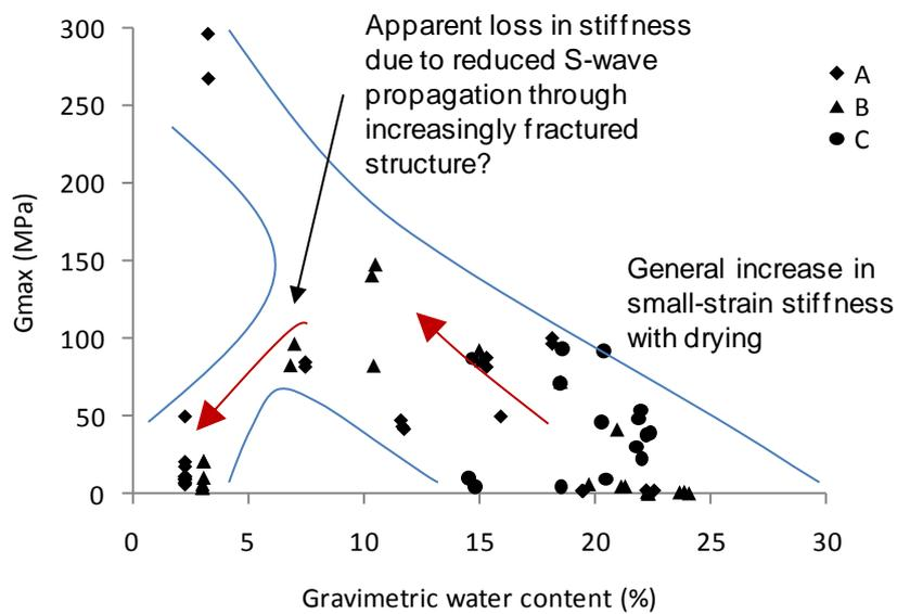
Figure 8 Small-strain shear modulus change with drying.
