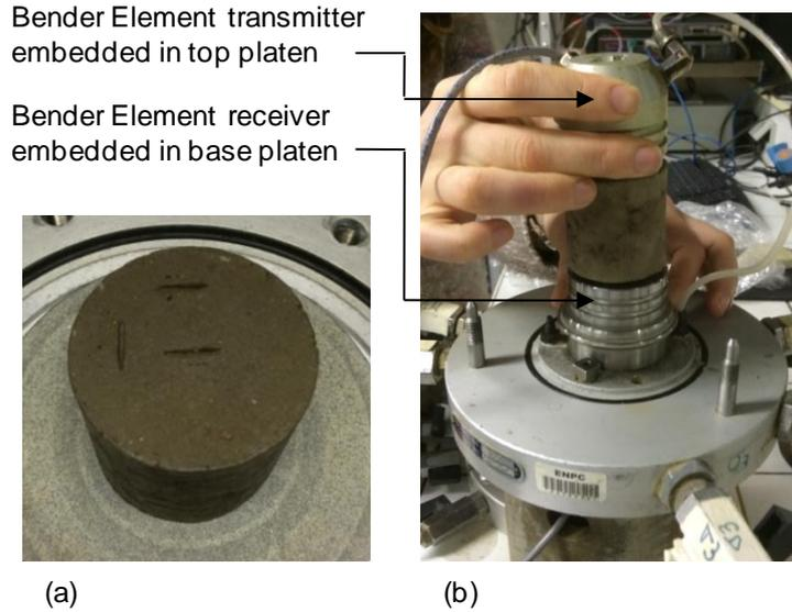
Figure 6 Bender Element experimental setup (a) sample showing three element impressions and (b) sample positioned between platens during testing.
