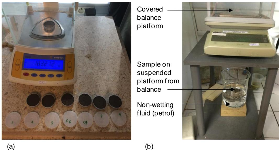
Figure 1 (a) WP4 samples drying to predetermined masses/moisture contents and (b) determination of sample density apparatus.
