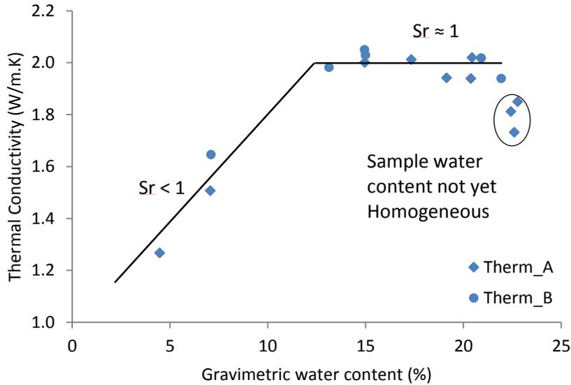
Figure 5 Thermal conductivity measurements at reducing sample masses due to drying
