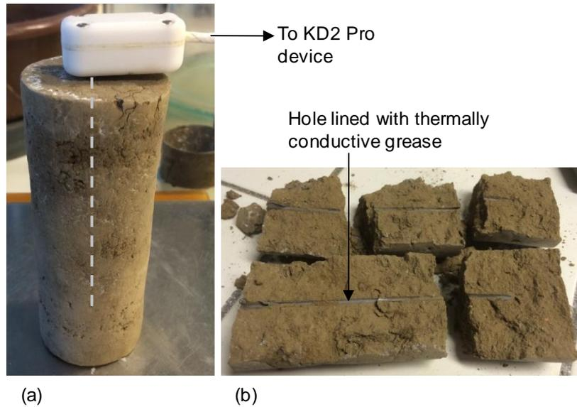
**Figure 4 Thermal conductivity testing setup (a) probe inserted into relatively dry, intact sample and (b) sample broken for moisture determination showing lined hole.**
