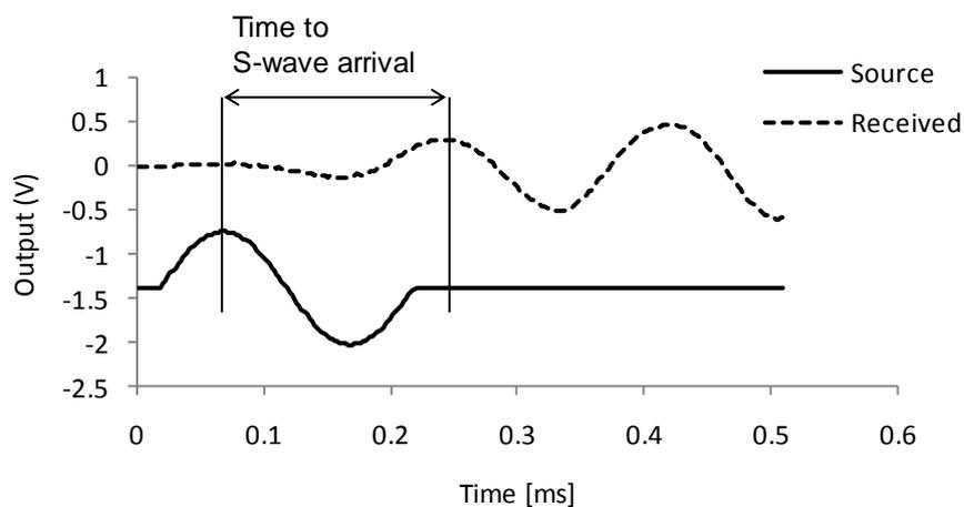
Figure 7 Example S-wave response at  $w = 12\%$ .
