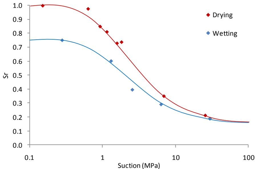
**Figure 2 SWRC for initial drying and single wetting path**
