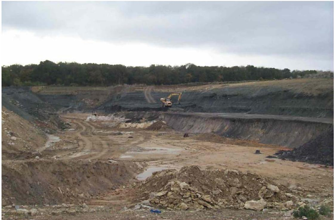
**Figure 3. Dark grey mudstone overburden is stripped from pale grey silty refractory clay at the Nassington Quarry operated by Vesuvius (UK) Ltd.**
